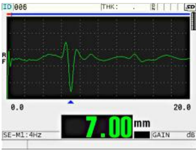
Typical conveyor belt measurement with M1036
